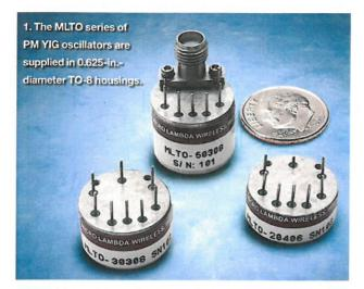
To accomplish wideband FM with these different magnet structures, different design approaches and different FM driver configurations were required. For an end user, the results are the same, with FM tuning coils capable of 3-dB bandwidths in excess of 20 MHz and with standard FM coil sensitivity the same for the two YIG oscillator types, at 150 kHz/mA. For either type of oscillator and FM coil, the minimum frequency deviation is ±15 MHz.
